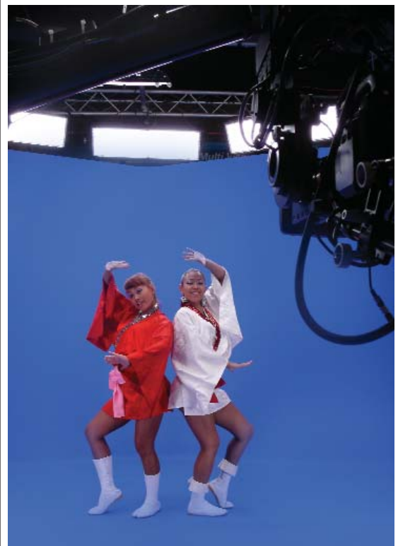
Image fixtures globed with 3200K lamps lighting virtual studio background, as well as dancers in the foreground.
