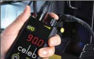
The dimmer knob on the remote dimmer adjusts the dimming. Press the dimmer knob to change the dim mode from **Coarse** to **Fine**. Coarse mode adjusts dimming in one rotation of the knob. In **Fine** mode, it will require 8 rotations for full range of dimming.
