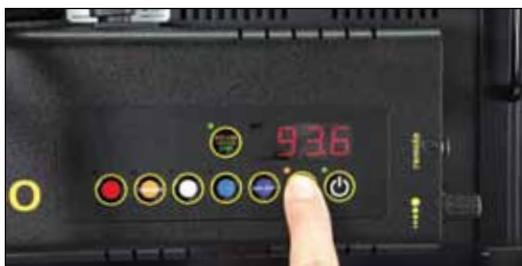
Press the **LOCK / RESET** button to lock the Kelvin and Dim settings. An amber indicator will display in **LOCK** mode.
