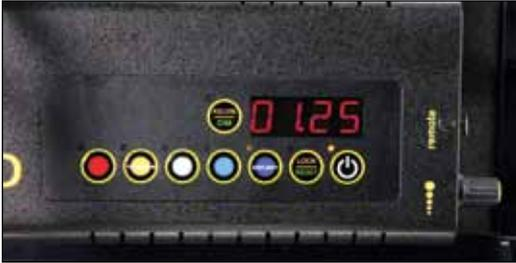
When power is first applied to the fixture, the alphanumeric display shows the current software version and date.
