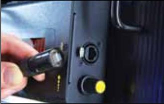
Insert the dimmer cable into the receptacle marked **REMOTE**. Insert the other end of the dimmer cable into the Remote Dimmer (**DIM-CE1**).
