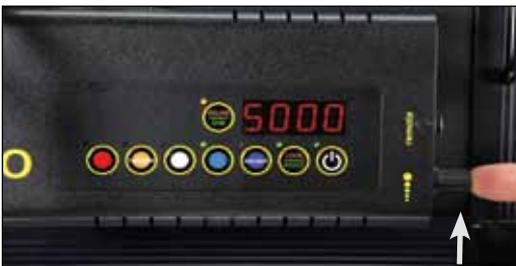
Press the rotating knob once to shift the Kelvin profile from Coarse to Fine increments.
