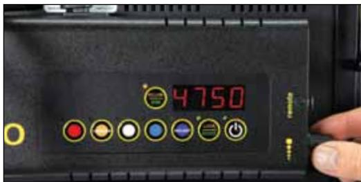
In **KELVIN** mode, the Kelvin can be fine tuned with the adjustment knob to any custom settings between 2700 to 5500.
