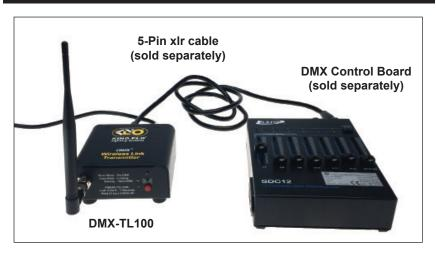
Connect the 5-pin xlr to the "**Out**" port of the DMX Control Board. Insert the 5-pin xlr cable into the "**In**" port of the DMX-TL100.
